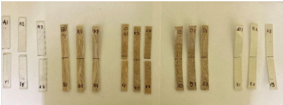
Figure 7. Condition of specimens after bending test
