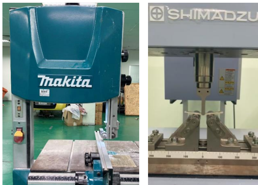
Figure 5. Band saw and universal testing machines with bending test setup
