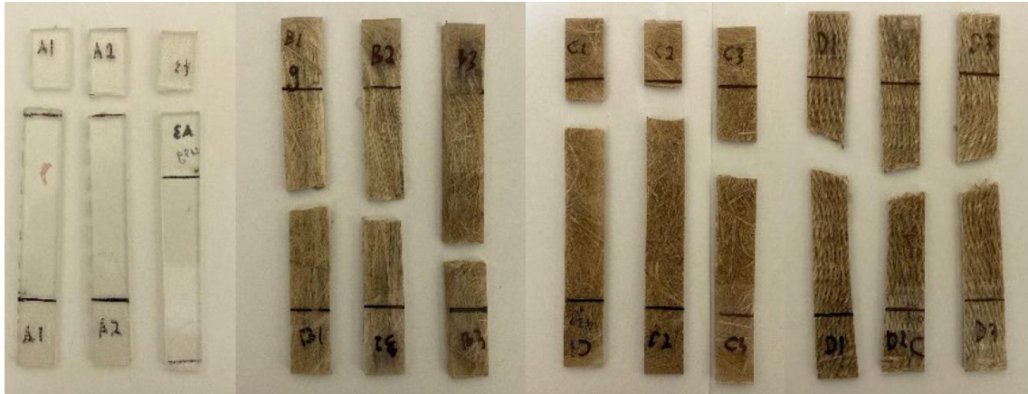
Figure 6. Condition of specimen after tensile test
