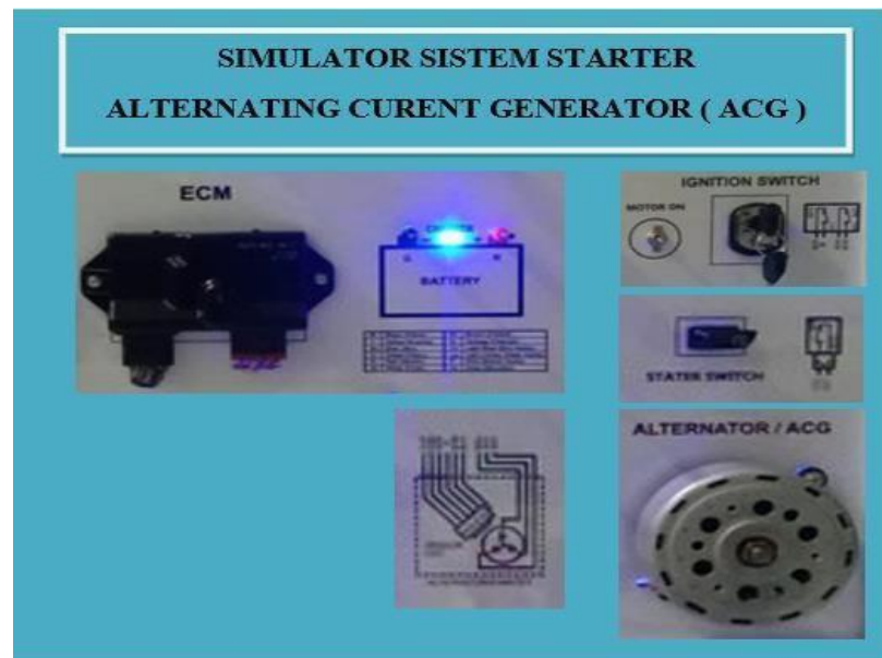
Gambar 8 Rancangan Simulator Kelistrikan System Starter ACG ( Alternating Current Generator )
