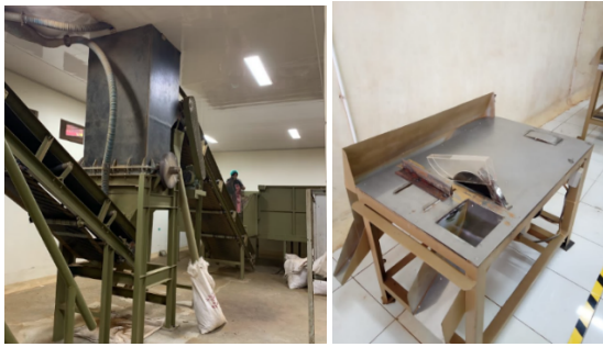
(a) (b) Gambar 2. Mesin broken and clean (a) Mesin potong (b)
