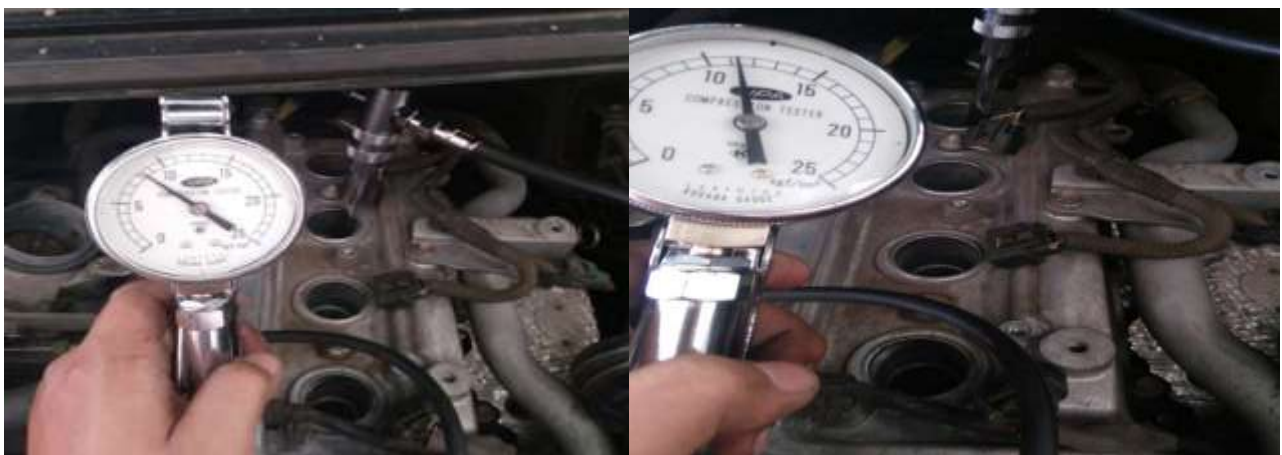
Figure 8 Results of Pressure Compression Checks on Cylinder & Results of Pressure Compression Checks on Cylinders (Source: 2018 Research Documentation)
