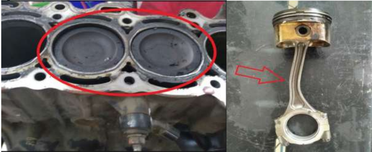
Figure 9 Difference in Torque Height when Upper Dead Point & Damage to the piston rod due to water hammer (Source:2018 Research Documentation)
