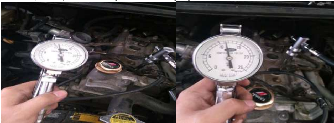
Figure 7 Results of Compression Pressure Checks on Cylinder & Pressure Compression Checks on Cylinder (Source: 2018 Research Documentation)
