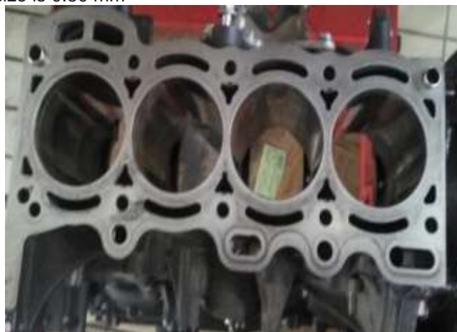
Figure 11. Cylinder Block After Oversize (Source: 2018 Research Documentation)
